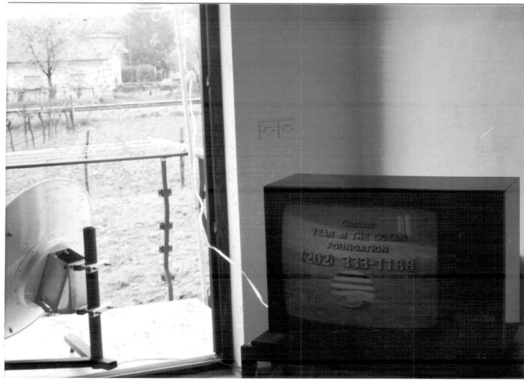
Fig. 5. - "Cable Network News" received with the 90cm dish
