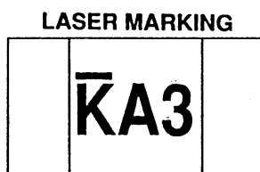
Example shown is a 1,000 pF capacitor.
