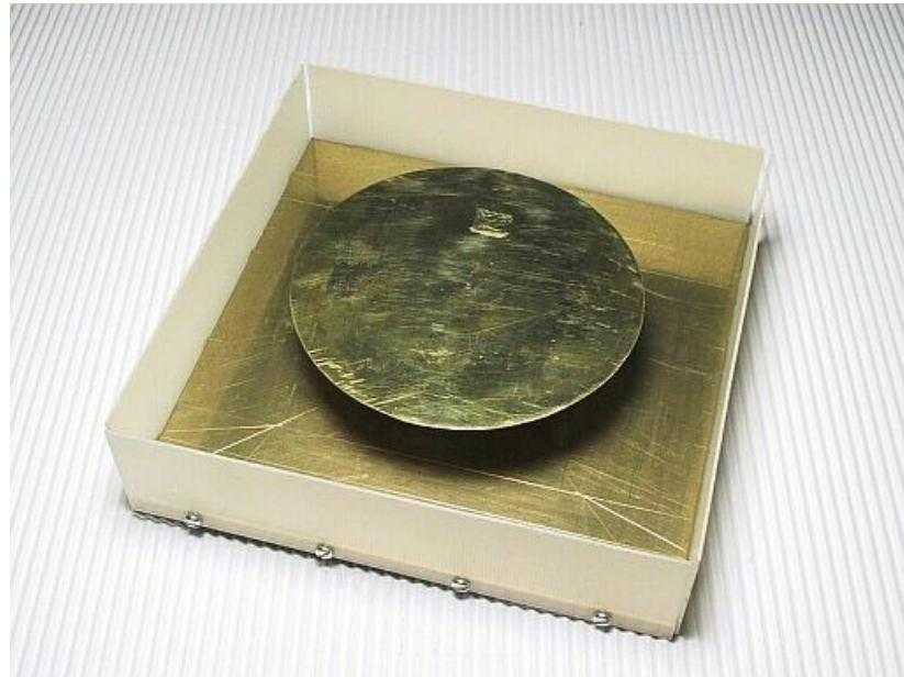
Practical experiments using this antenna with both an ATC transponder and with a DME (same frequency band) gave excellent results. Thanks to its gain, this antenna can fully meet the ICAO specifications with a transponder output power of only 25W.
