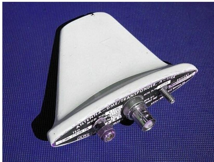
The antenna is shaped as a fin to reduce aerodynamic drag. A blade antenna has a gain of around 2dBi when installed correctly on a large metal ground plane. This antenna is therefore suitable for installation on metal fuselages. In the case of composite fuselages, the antenna requires an additional sheet of metal to act as a ground plane.
