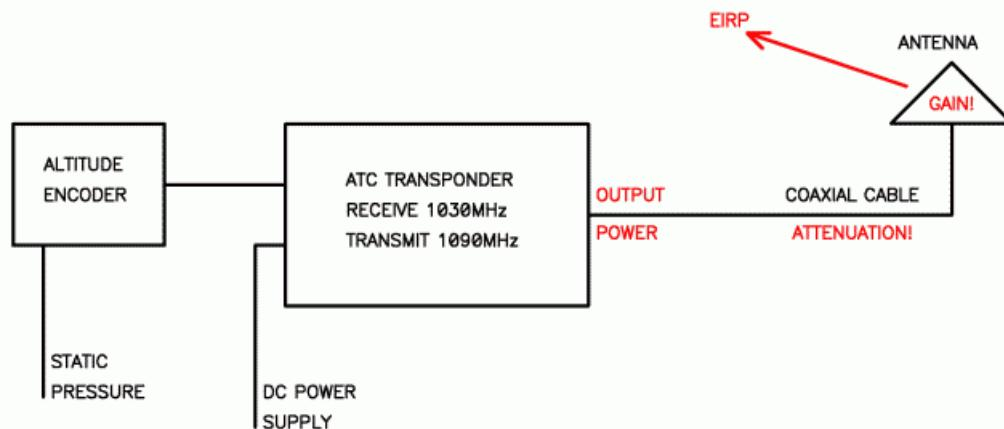
What is the required power of an ATC transponder? ICAO specifies the Effective Isotropic Radiated Power (EIRP), therefore considering the output power of the transponder itself, the inevitable power losses due to antenna-cable attenuation and an eventual antenna gain. The peak (pulsed) EIRP should be between 125W (+21dBW) and 500W (+27dBW). The lower EIRP limit is further reduced to 70W (+18.5dBW) for aircraft flying below FL150.
