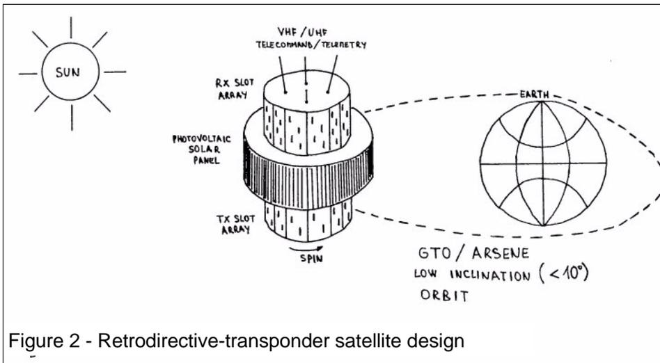
Due to the spin stabilization, the antenna beams need to be counterrotated to track the user groundstations. Therefore the antenna beam only needs to be steered in one dimension in the equatorial plane, while the single array elements can already provide a suitable radiation pattern in the north-south plane. Very suitable antenna elements are waveguide slot arrays.
