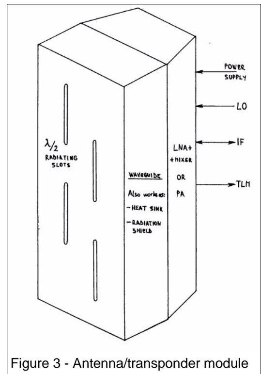
Figure 3 - Antenna/transponder module
