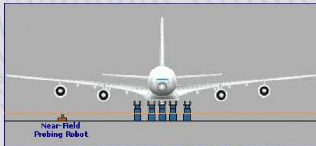
Ground (Vehicle) Scanners for Horizontal Planar NF-Scans under the Aircraft
