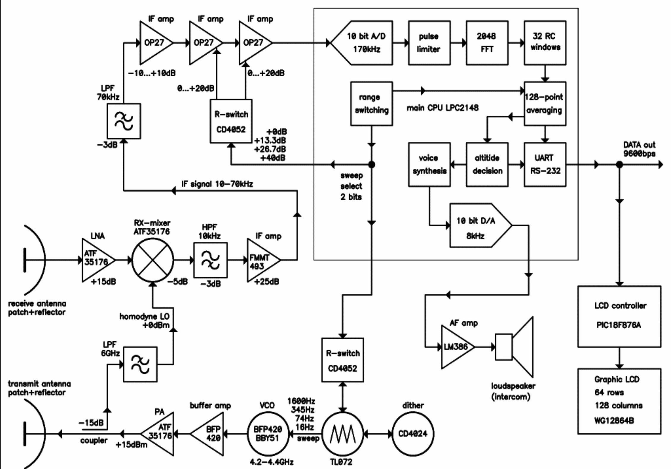
Airborne RADAR: 4.3GHz, 30mW, 1.5km range, dual antenna
