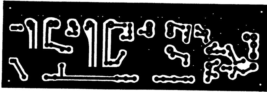
Fig. 3 - TX exciter PCB (single-sided 0.8mm glassfiber-epoxy).
