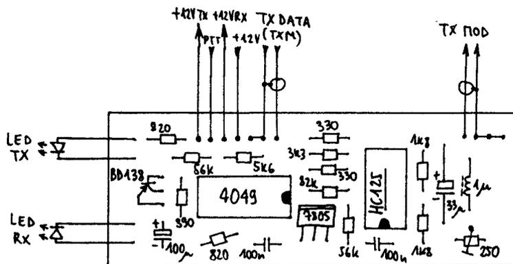
Fig. 25 - Supply switch interface component location.
