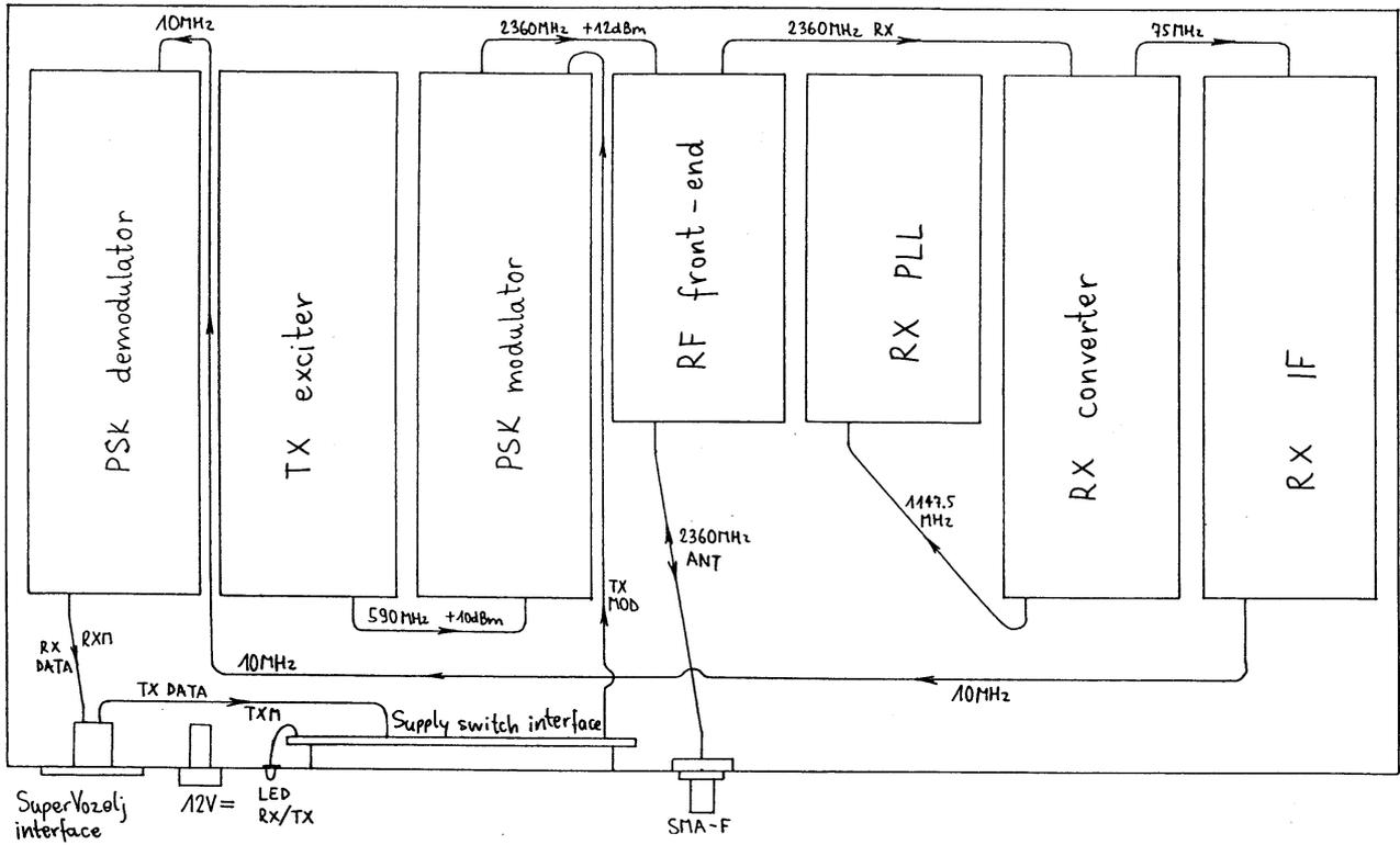
Fig. 26 - 13cm PSK transceiver module location.
