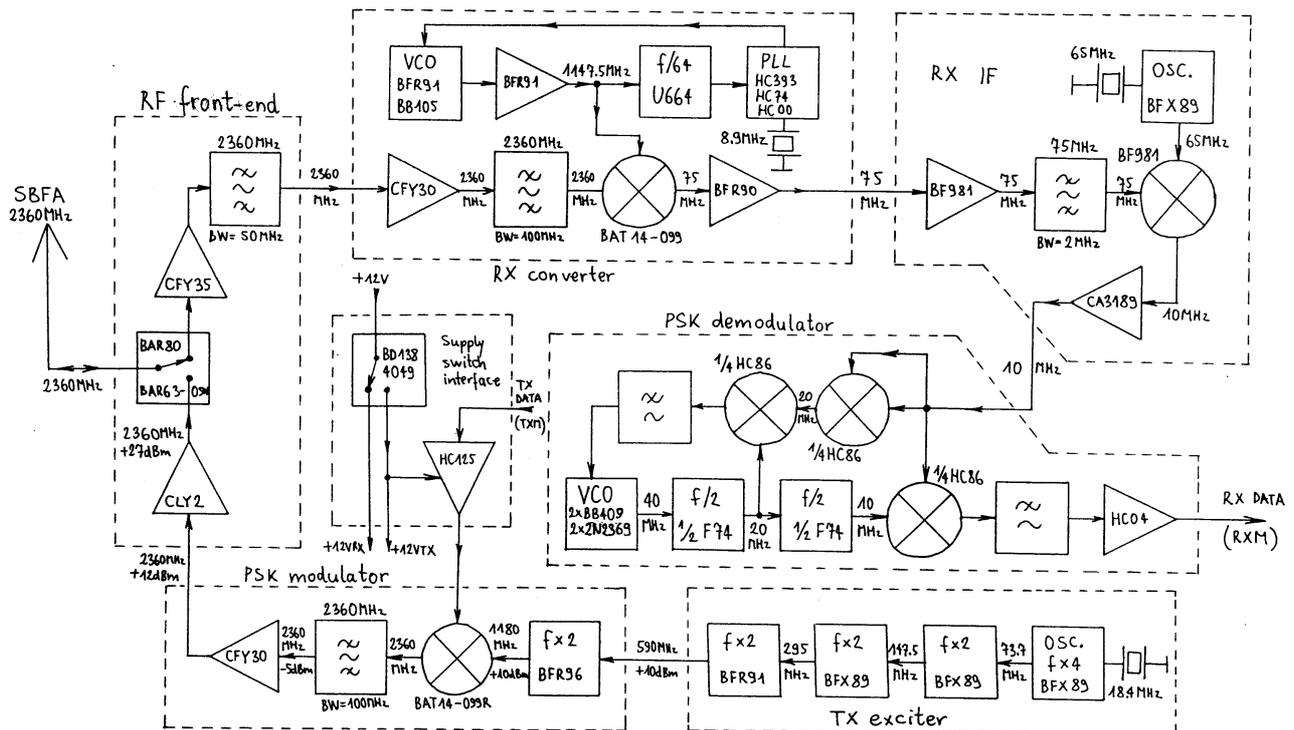
Fig. 1 - 13 cm PSK transceiver block diagram (2360MHz / 1.2288 Mbit/s).
