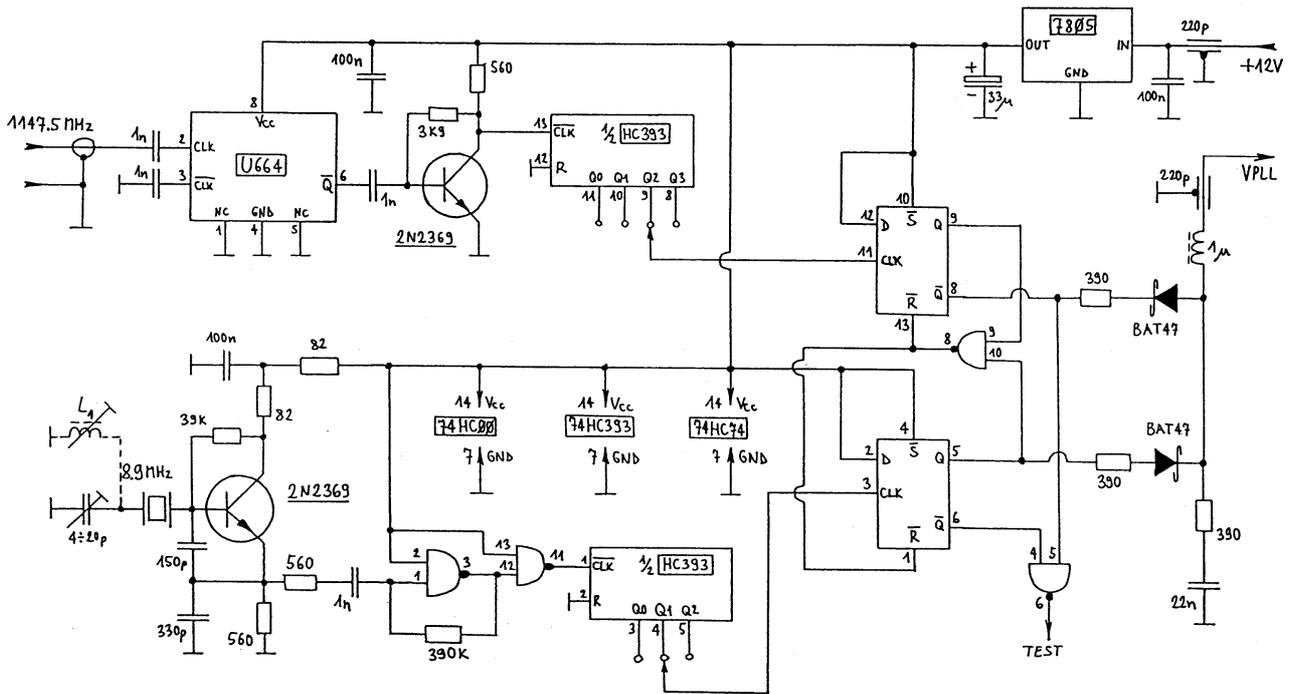
Fig. 14 - RX converter, PLL circuit diagram.
