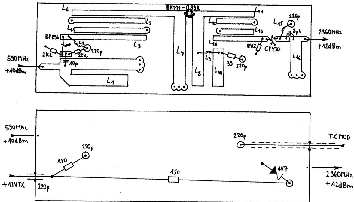
Fig. 7. - PSK modulator component location.
