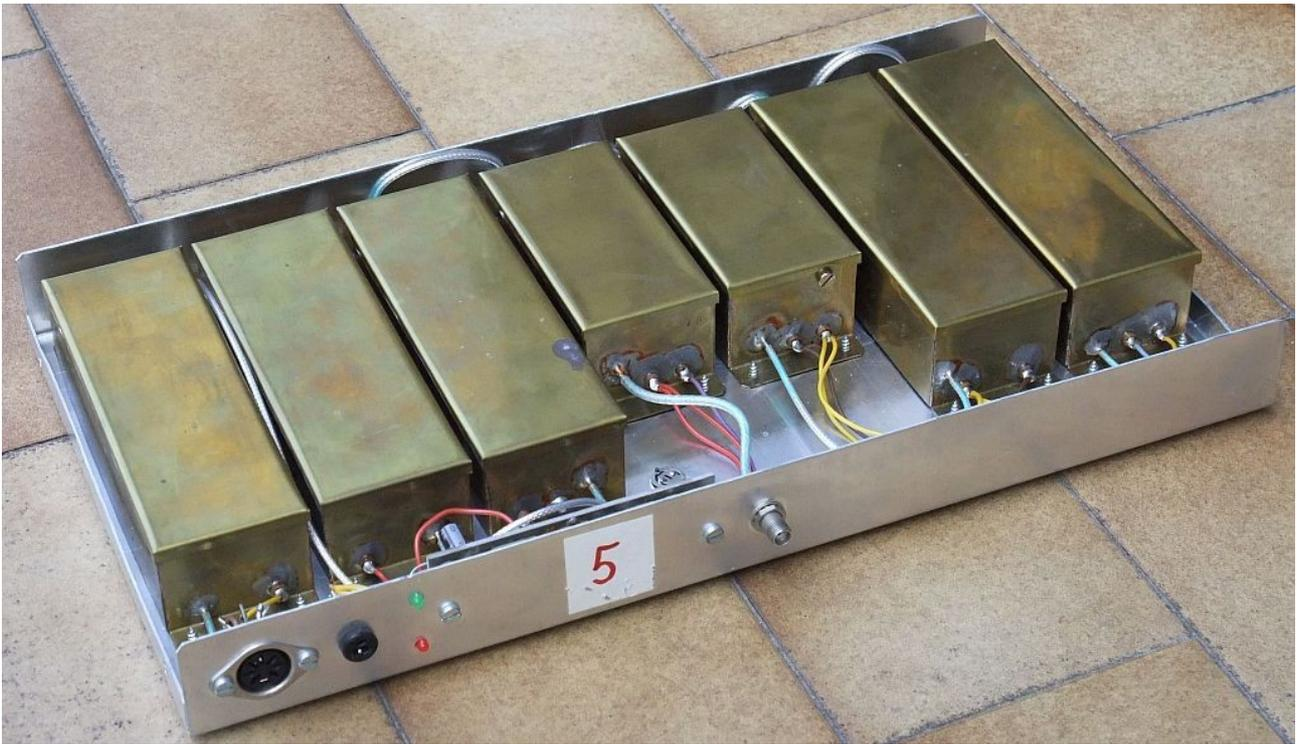
To retain the shielding efficiency of the single modules, all of the supply and low-frequency interconnects go through 220pF feed-through capacitors soldered in the narrow sides of the brass frames. The RF interconnects are made with thin 50-ohm teflon cables (RG-188 or similar). It is extremely important that the coax shielding braid is soldered in a "watertight" fashion to the brass sheet all around the central conductor using a suitable soldering iron.
