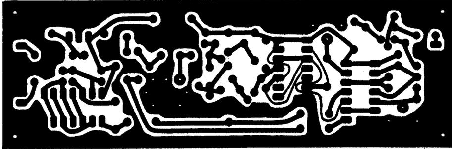
Fig. 21 - PSK demodulator PCB (single-sided 1.6 mm glassfiber-epoxy).
