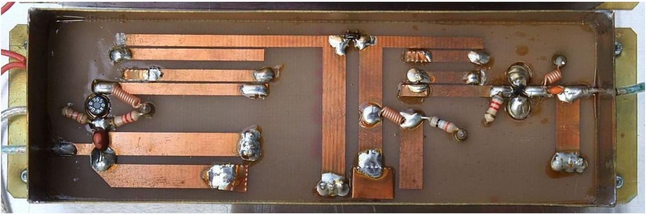
Although most of the transmission lines are etched on the PCB, L2, L9 and L15 are air-wound quarter-wavelength chokes. L2 is a quarter-wavelength choke for 1180MHz, L15 is a quarter-wavelength choke for 2360MHz while L9 should be a quarter-wavelength somewhere in the middle (around 1700MHz), since it has to be effective for both frequencies.
