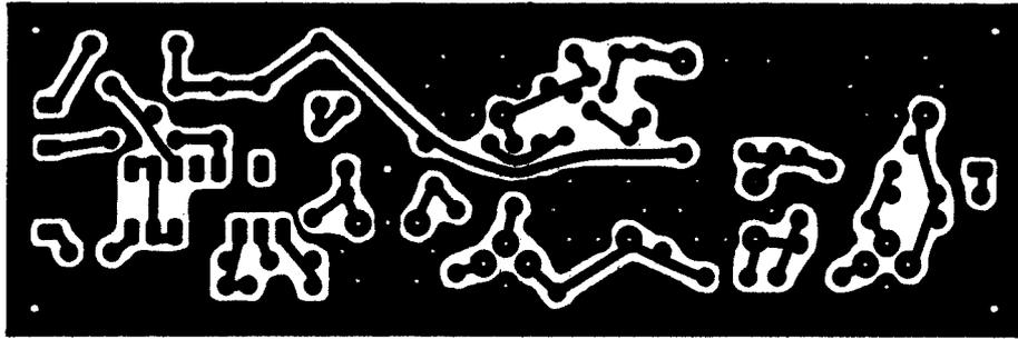
Fig. 18 - RX IF PCB (single-sided 1.6 mm glassfiber - epoxy).
