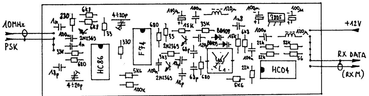
Fig. 22 - PSK demodulator component location.
