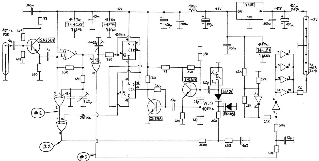
Fig. 20 - PSK demodulator circuit diagram.
