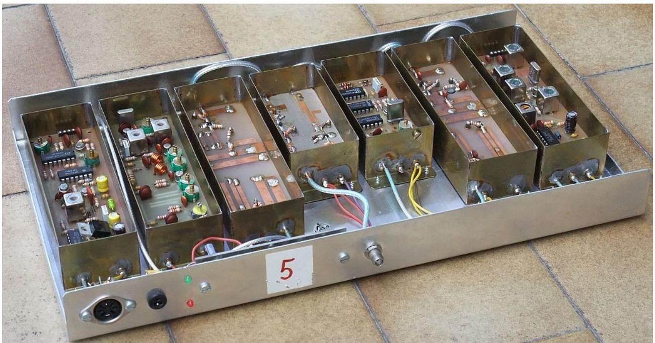
In this article a successful 13cm BPSK transceiver design will be described. In the 13cm amateur band, the sum of the frequency uncertainties of both receiver and transmitter is at least 10kHz using top quality temperature-compensated crystal oscillators. A real-world figure is 100kHz frequency uncertainty that requires a MINIMUM bit rate of about 1Mbit/s!
