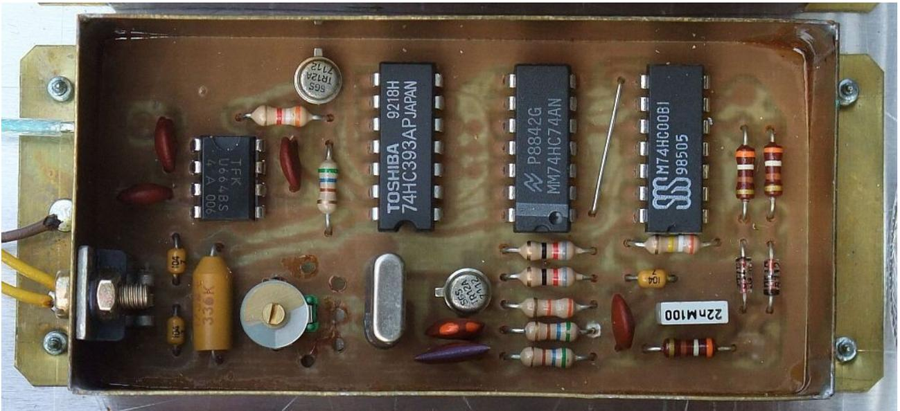
The only adjustment of the PLL is to bring the crystal oscillator to the required frequency. The PLL lock test point is not brought out of the shielding enclosure since it is only required during the adjustment of the PLL.
