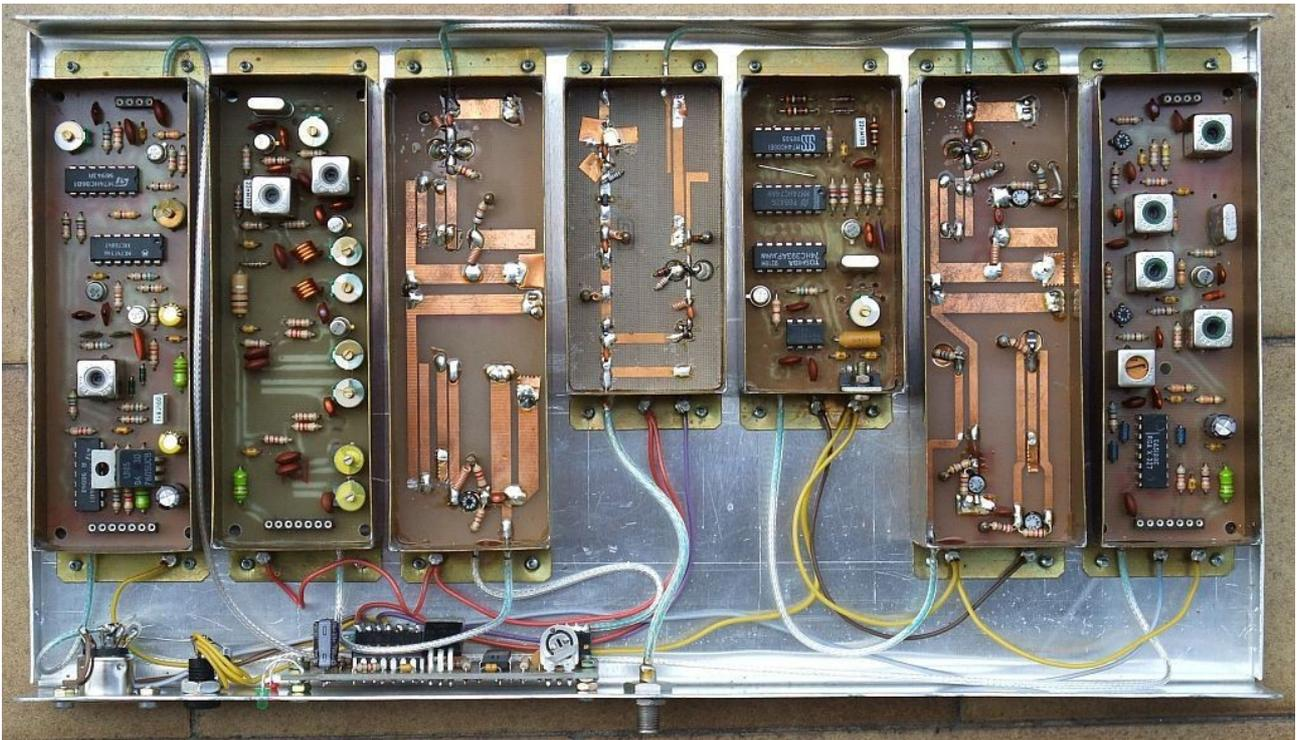
The PSK transceiver is enclosed in a custom-made aluminum box measuring 320mm (width) X175mm (depth) X32mm (height). The individual module locations and RF interconnects are shown on Fig.26. The box is made of two "U"-shaped pieces of aluminum sheet. The front, bottom and back are made of 1mm thick aluminum sheet, while the cover and the two sides are made of 0.6mm thick aluminum sheet. The cover and sides are 190mm deep to exceed the size of the bottom by 7.5mm on the front and on the back.
