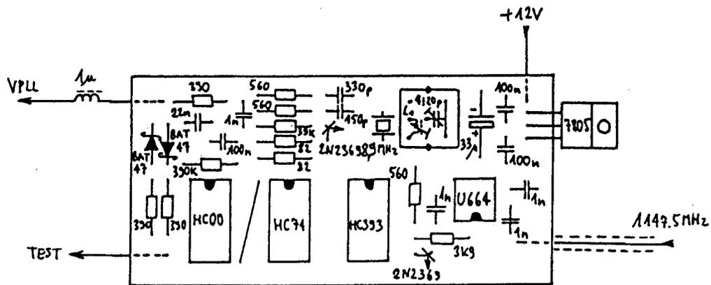
Fig. 16 - RX converter, PLL component location.
