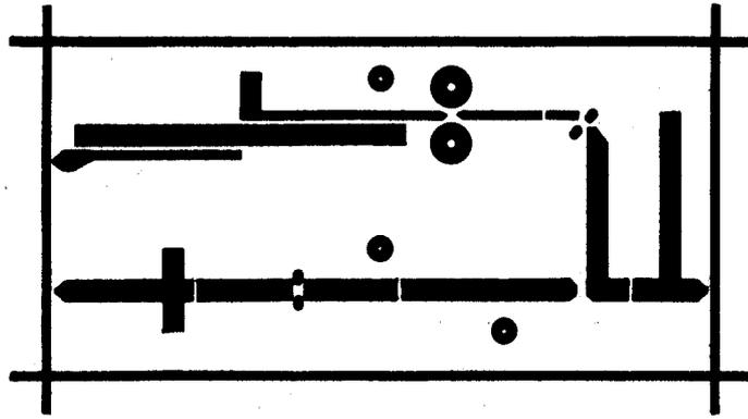
Fig. 9 - RF front-end PCB (double-sided 0.8mm glassfiber-teflon, microstrip circuit with a continuous ground plane).
