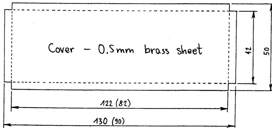
Fig. 27 - 13cm PSK transceiver shielded module enclosure.
