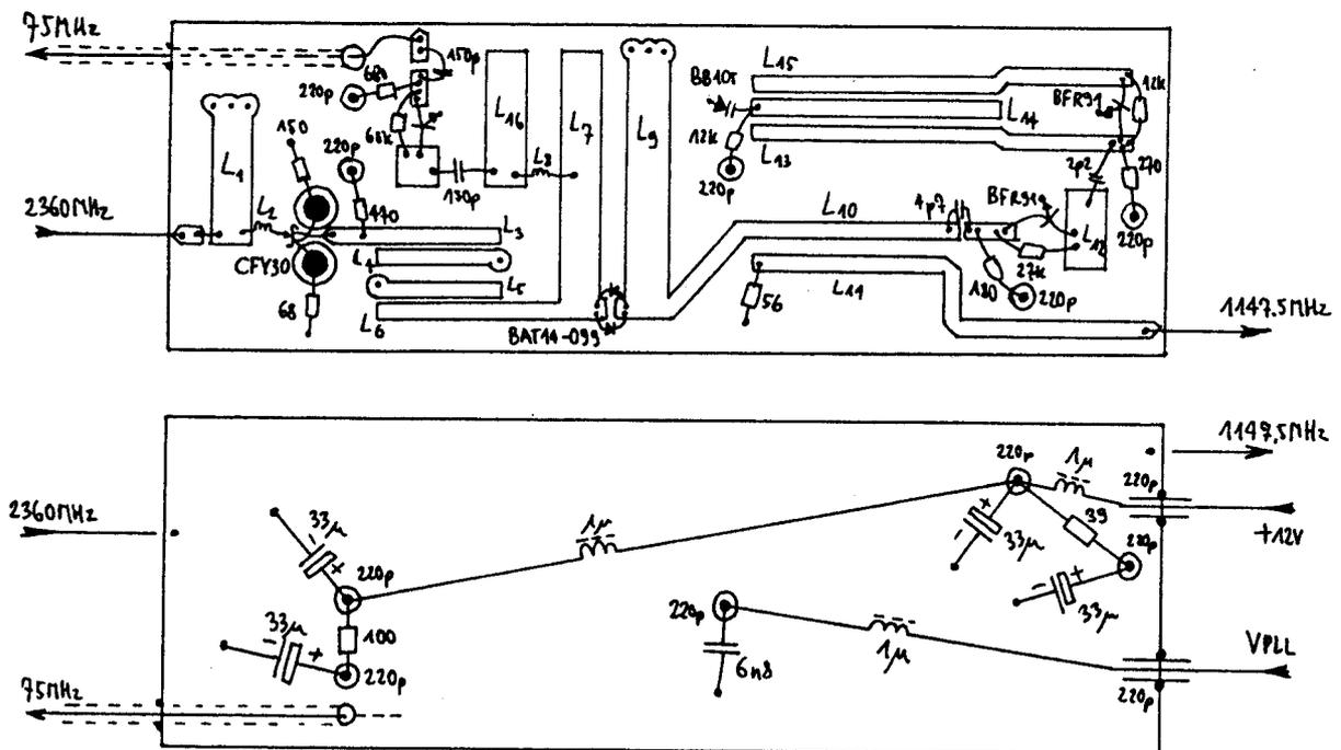
Fig. 13 - RX converter, analog section component location.
