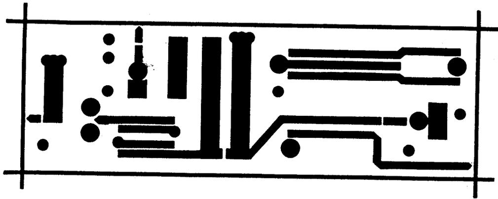
Fig. 12 - RX converter, analog section PCB (double-sided 1.6 mm glassfiber - epoxy, microstrip circuit with a continuous groundplane).
