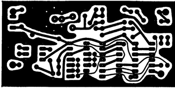
Fig. 15 - RX converter, PLL PCB (single-sided 0.8mm glassfiber-epoxy).
