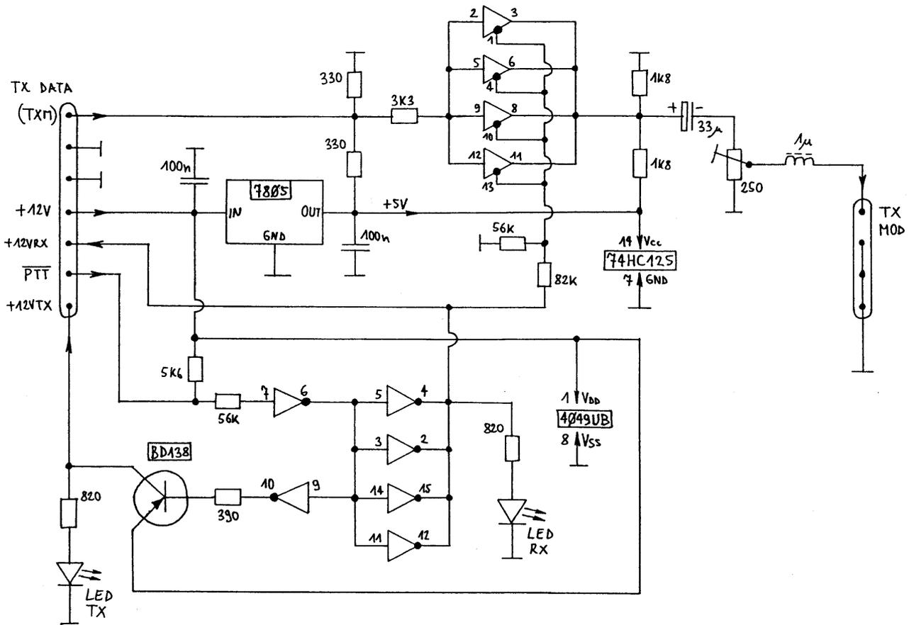
Fig. 23 - Supply switch interface circuit diagram.
