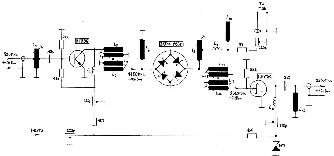
Fig. 5 - PSK modulator circuit diagram.
