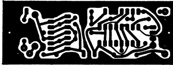
Fig. 24 - Supply switch interface PCB (single-sided 1.6 mm glassfiber - epoxy).
