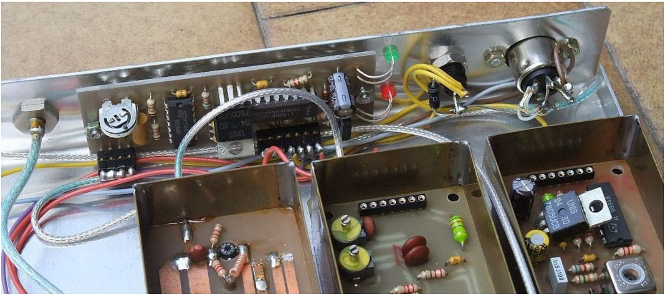
10. Assembly of the 13cm PSK transceiver
