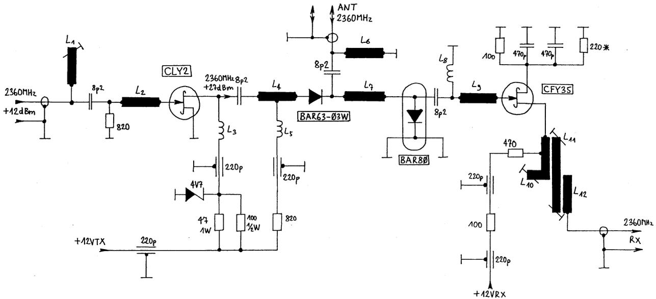
Fig. 8 - RF front-end circuit diagram.
