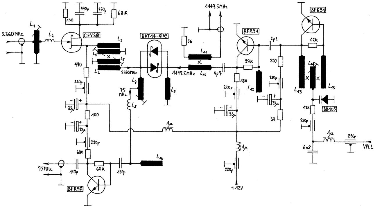
Fig. 11 - RX converter, analog section circuit diagram.
