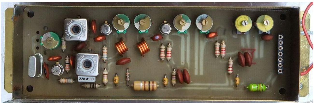
L2 and L3 have about 150nH each or 4 turns each of 0.25mm thick copper-enameled wire. They are wound on 36MHz (TV IF) coil formers with a central adjustable ferrite screw, plastic cap and 10mmX10mm square shield. L4 and L5 are self-supporting coils with 4 turns each of 1mm thick copper-enameled wire, wound on an internal diameter of 4mm. Finally, L6, L7, L8 and L9 are etched on the
