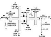
required on the RF side of the mixer since the quarter-wavelength LO traps behave as half-wavelength resonators at the input RF.
