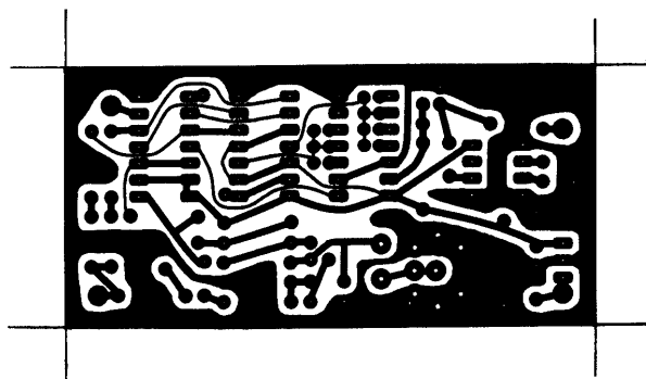
Fig. 8. - Printed-circuit board for the 2.4 GHz converter, PLL logic, single-sided, bottom view.
