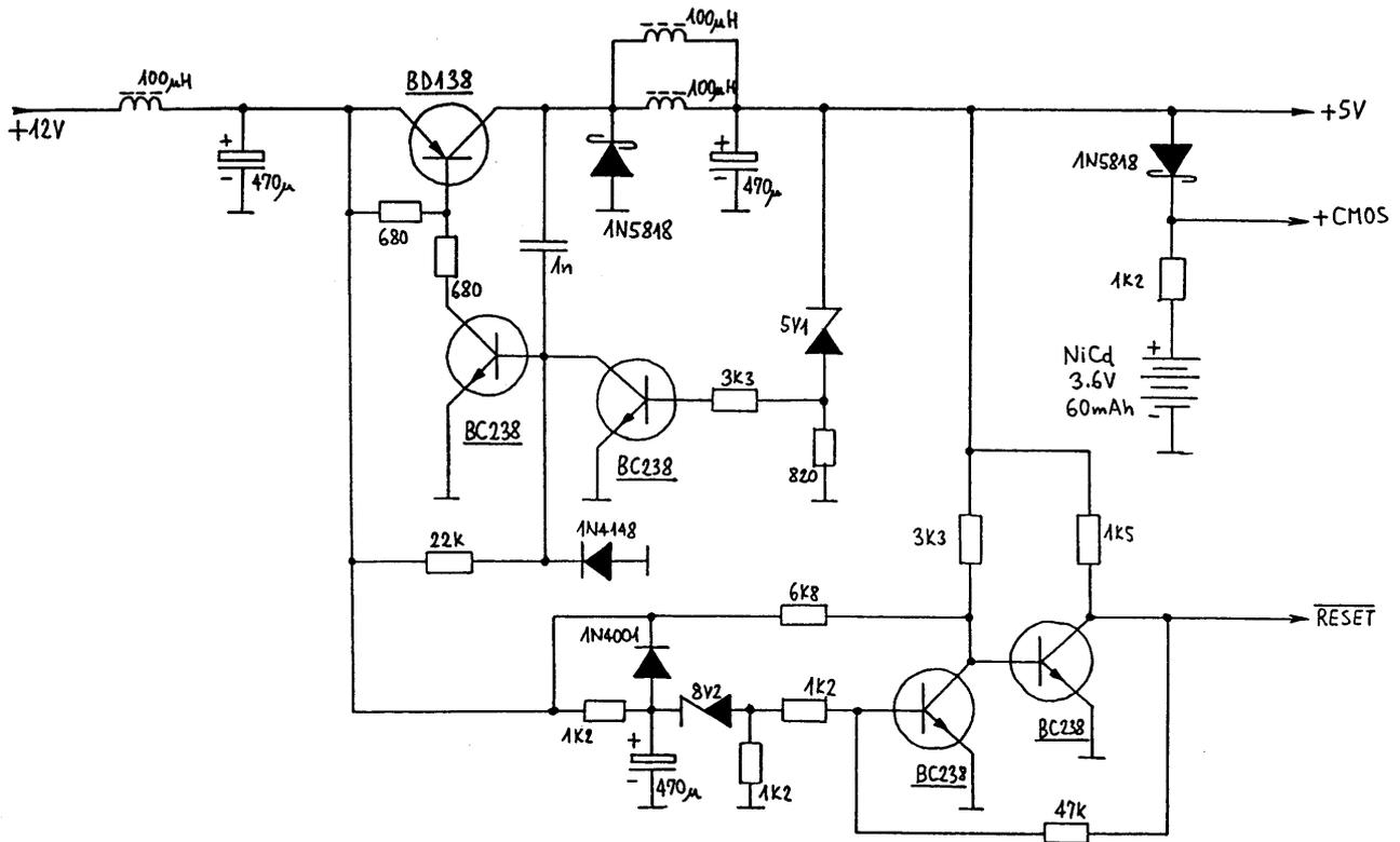
Fig. 9 - Power supply and reset circuit.
