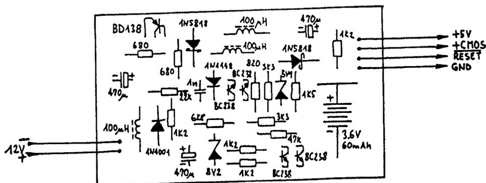
Fig. 11 - Power-supply component location.
