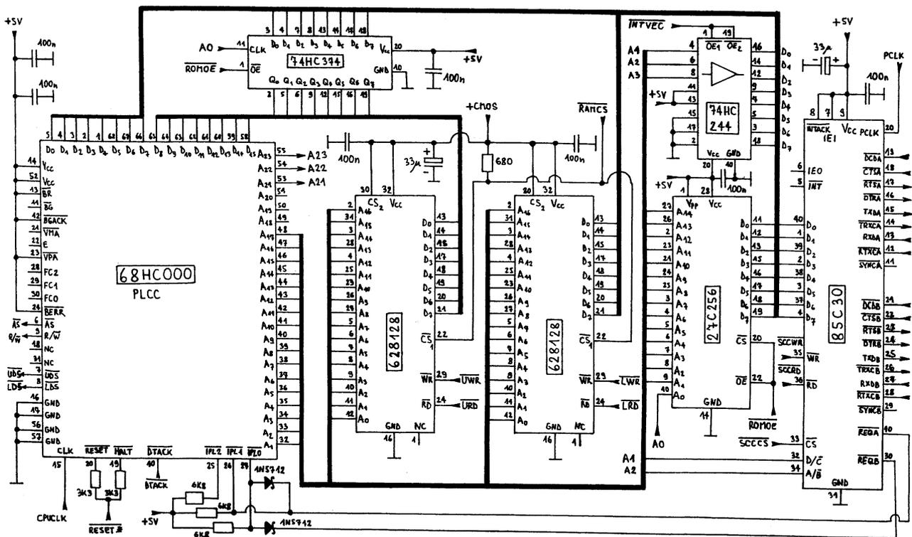
Fig. 1 - CPU, memory and serial port.
