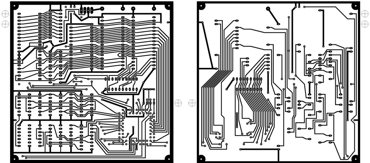
Fig. 3 - TNC double-sided printed-circuit board.
