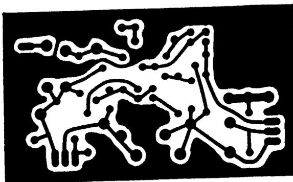
Fig. 10 - Power-supply printed-circuit board.
