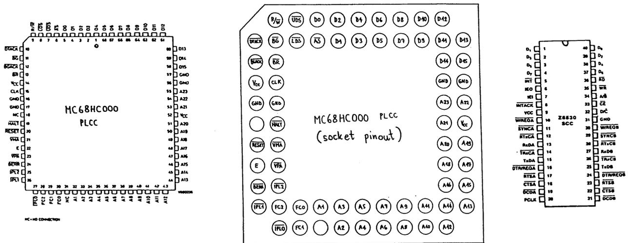
Fig. 5 - CPU and serial-port pinouts.
