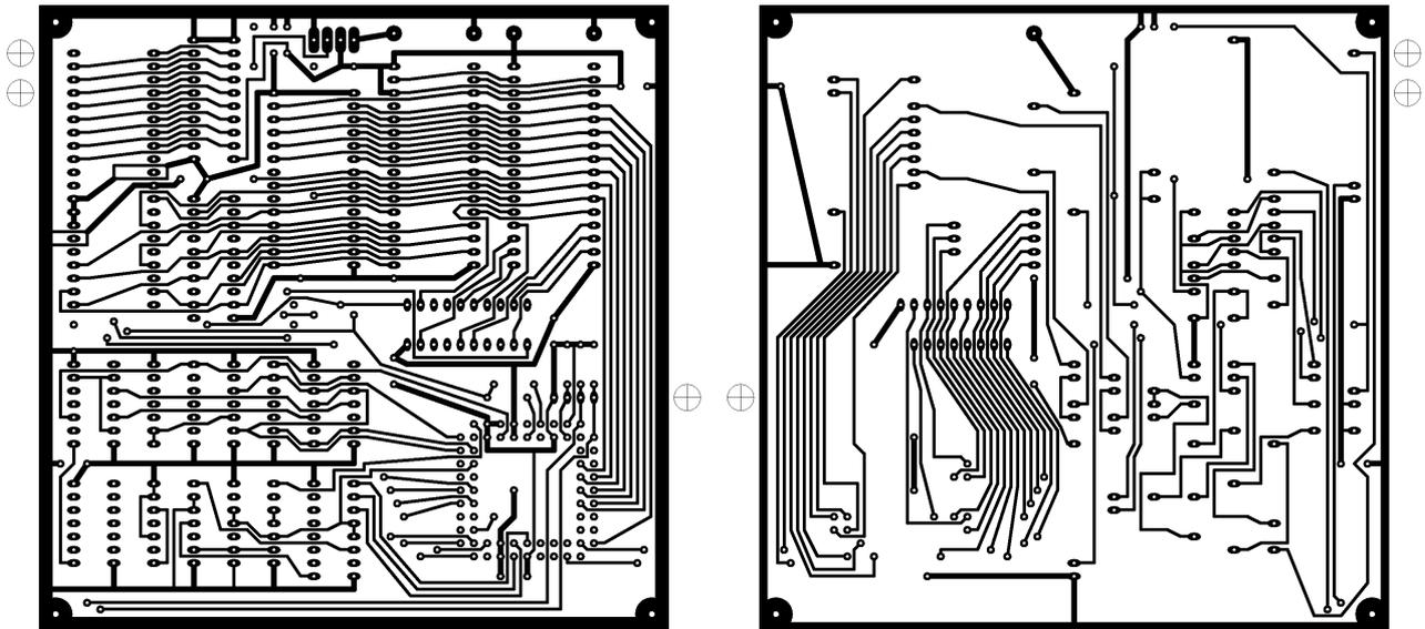
Fig. 3 - TNC double-sided printed-circuit board.
