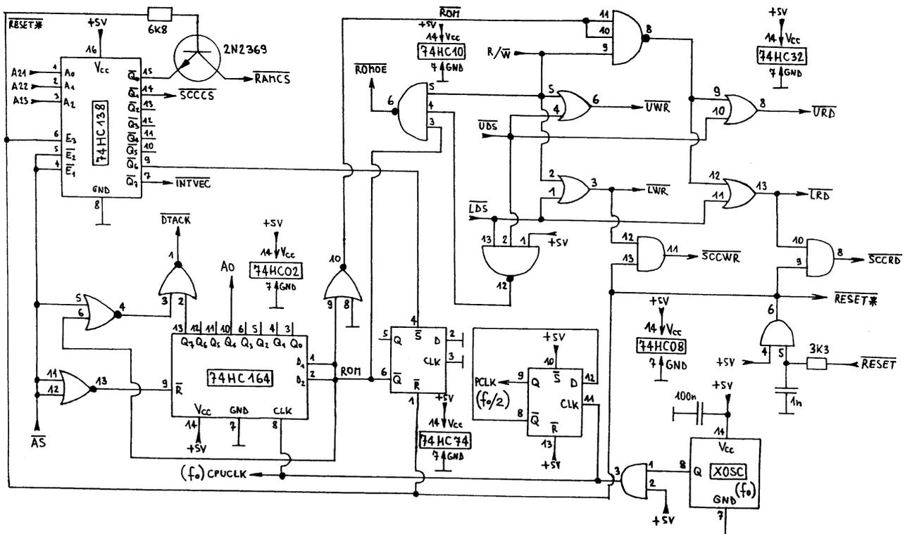
Fig. 2 - Bus interface logic.
