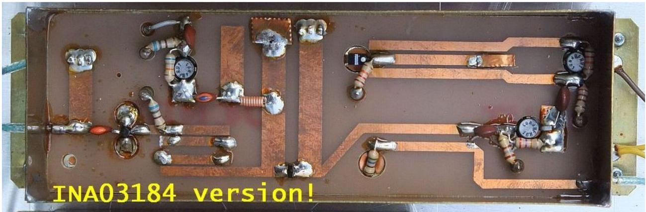
An alternative solution is to replace the CFY30 GaAs FET with the silicon MMIC INA-03184. The latter has a higher noise figure but offers more gain and does not self oscillate. When using the INA-03184, L2 has to be replaced with a 6.8pF capacitor, the output bias resistor has to be increased from 470ohm up to 680ohm and the source bypass capacitors and bias resistors are no longer required, since the two INA-03184 common pins can be grounded in a straightforward way.
