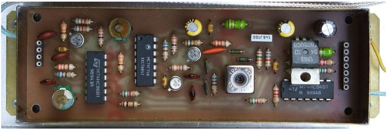
The alignment of the PSK demodulator should start with the adjustment of the delay of the input signal frequency doubler. A DC voltmeter is connected to test point #1 through a RF choke. The capacitive trimmer on pin 5 of the 74HC86 is adjusted to obtain an average (DC) voltage of 2.5V on test point #1 with some input signal: either receiver noise or a valid PSK signal.
