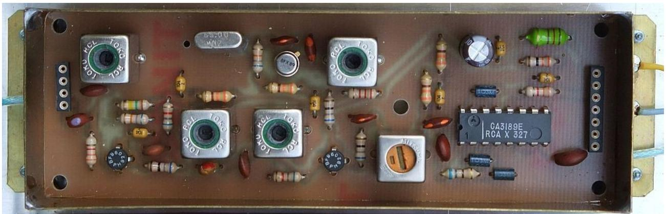
The IF chain alignment should start by checking the operation of the 65MHz crystal oscillator on the desired overtone and adjusting L4 if necessary. All other tuned circuits (L1, L2, L3 and L5) are simply aligned for the maximum gain. Since the same circuits also define the selectivity of the receiver, the alignments have to be performed using a suitable 75MHz signal source: signal generator or grid-dip meter. The receiver thermal noise or other noise sources can not be used for this purpose.
