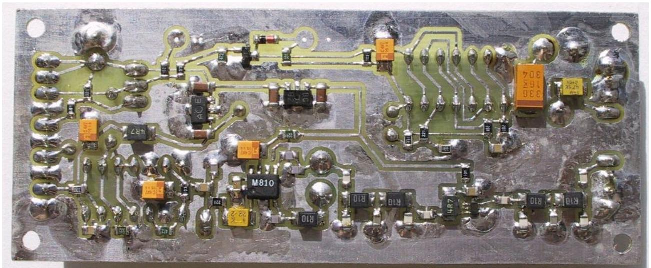
Both microwave boards are microstrip circuits (25mmX80mm and 20mmX80mm) built on 0.5mm (19mils) thick Ultralam 2000 teflon laminate. The remaining boards (twice 20mmX80mm and 40mmX100mm) are single-sided FR4:
